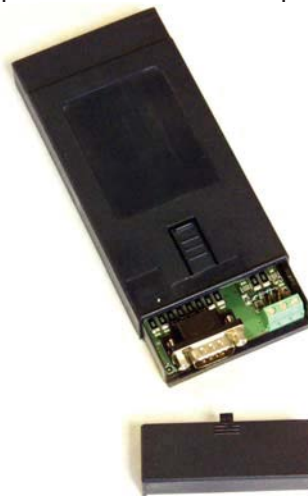
Figure 6: Expansion module with exposed connectors
